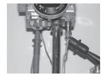
Step 3. If continuity is indicated, the ECO is OK. If continuity is not indicated, the ECO has opened and the combination thermostat/gas valve must be replaced.
